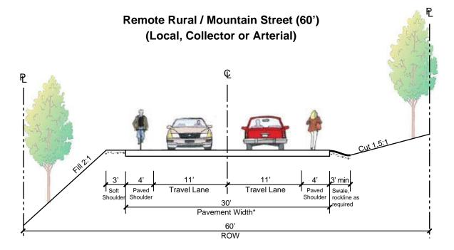
\* Desired dimensions shown. If terrain requires reduction in width, give priority to shoulders in uphill direction.
